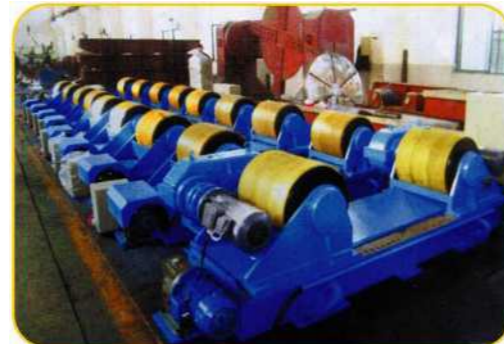
可调 250T 宽轮 (聚氨酯轮) 250T Welding Rotators (With Wide Polyurethane Wheels)
